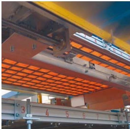
Quartz heating elements for fast, efficient heating of plastic sheets
